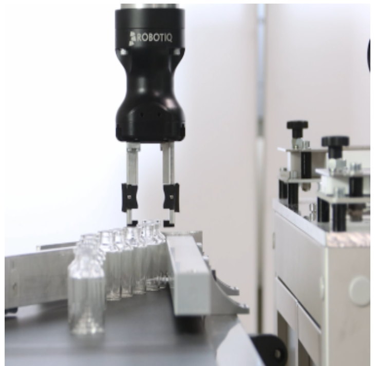
Conveyor belt pick-up
