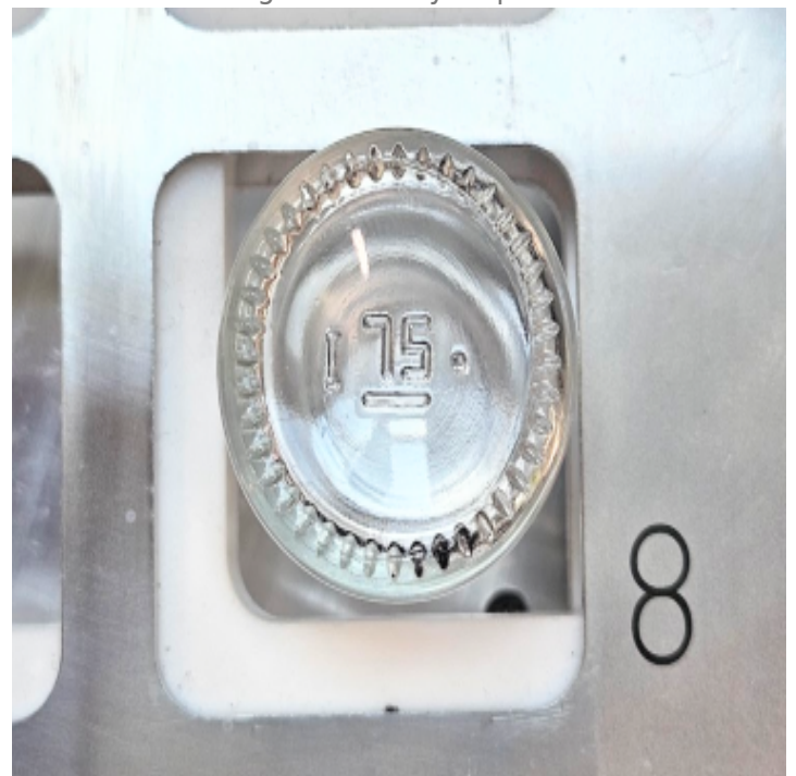
Dotcode cavity inspection
